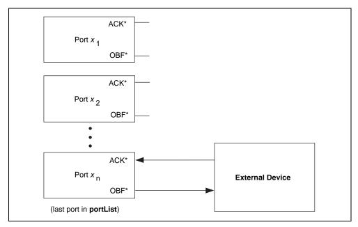
Figure 2-13. Digital Scanning Output Group Handshaking Connections
